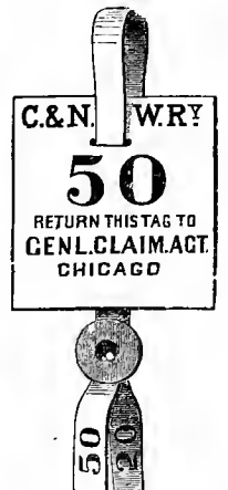
Fig. 3884. TIN SHACKLE AND LEAD SEAL WITH TIN RETURN-TAG.
